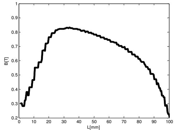
Fig. 5 Magnetic flux density along the rotor pole
