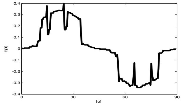
Fig. 10 Magnetic flux density in the air-gap along a pole-pair of the third structure
