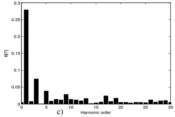
Fig. 12 Air-gap magnetic flux density spectrum: a) first structure, b) second structure, c) third structure
