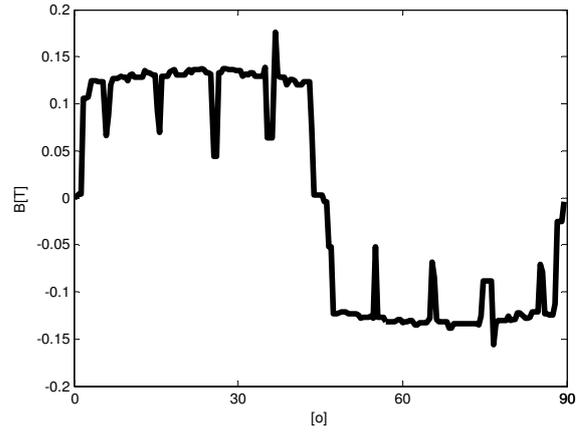
Fig. 3 Magnetic flux density in the air-gap along a pole-pair
