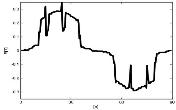
Fig. 8 Magnetic flux density in the air-gap along a pole-pair of the second structure
