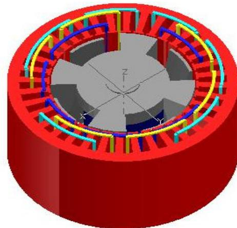
Fig. 1 3D view of the claw-pole PMSM
