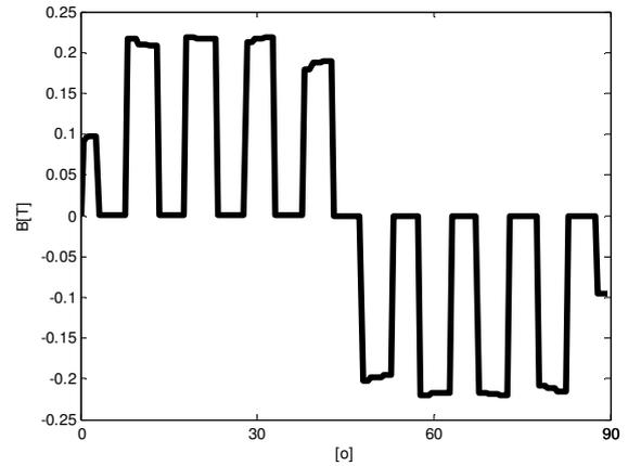
Fig. 4 Magnetic flux density in the stator teeth along a pole-pair
