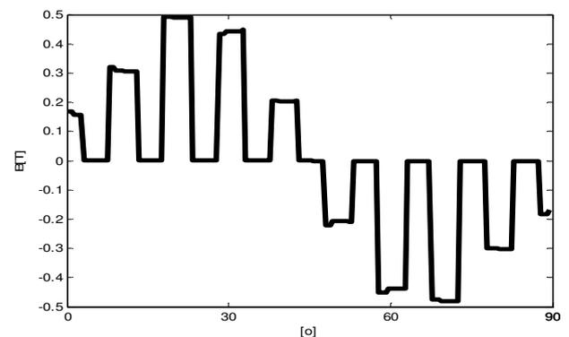
Fig. 11 Magnetic flux density in the stator teeth along a pole-pair of the third structure
